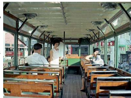
Seating on the tram was relatively spartan until the fleet was modernized in the 1980s. This 1966 view of the upper deck of tram No. 21 shows the standard wooden seating that was offered. At this stage, the upper deck was reserved for first-class passengers, who entered the tram via the front entrance, while the lower deck was occupied by third-class passengers, who entered via the rear platform. The two-class fare structure was abolished in 1972.
